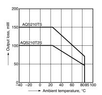
2. Relative output current vs. ambient temperature characteristics
