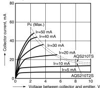
4-2. Collector current vs. voltage between collector and emitter characteristics (Ic-VcE) Measured portion: between terminals 6 and 7 (AQS210TS), (AQS210T2S)
