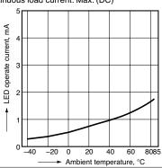
LED turn off current vs. ambient temperature characteristics
